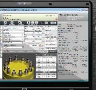
**Bolt Load Software** Takes the complexity out of tensioner and torque calculations.
