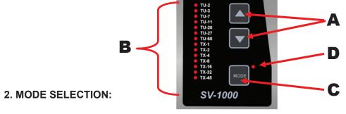
The mode selection button allows the user to operate the TLM ultrasonic device in conjunction with the SV series auto cycling pumps.
