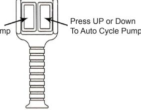
Press Either Button To Turn Pump On
