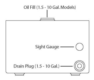
Run the pump in no load condition for 1 or 2 minutes maximum. Unplug the pump and remove the motor and pump assembly again. Now drain the flushing oil and re-clean the inside of the reservoir. (Make sure flushing fluid is also drained from pump assembly). Reassemble the pump and refill the reservoir with TorcUP hydraulic oil and reassemble the pump.
