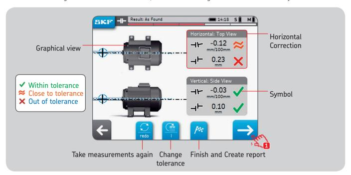
The black shafts icons are fixed and do not represent the alignment state.
