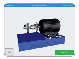
When the system senses that the shaft has been rotated sufficiently, and has been left untouched for a short while, it will automatically record the  $2^{nd}$  measurement position.
