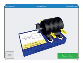
An animation shows the bolts being tightened down. Alignment is now complete and to confirm the result there is a need to re-do the measurement. Tap Remeasure.
