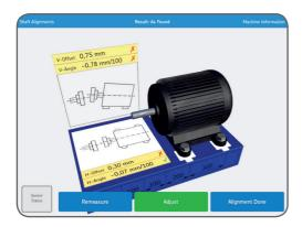
The values are compared with the selected tolerances and the symbols to the right, of the offset and angular misalignment values, indicate if the values are within tolerance.
