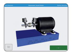
When the system senses that the shaft has again been rotated sufficiently, and has been left untouched for a short while, it will automatically record the 3<sup>rd</sup> measurement position.
