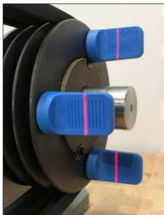
Fig.6 – Display of horizontal angle misalignment
