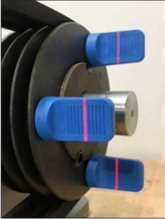
Fig.10 – Horizontal angle misalignment correction
