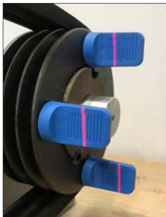
Fig.5 – Display of vertical angle misalignment
