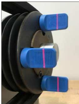
Fig.12 – Pulleys perfectly aligned
