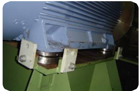
Details of the SKF Vibracon chock
